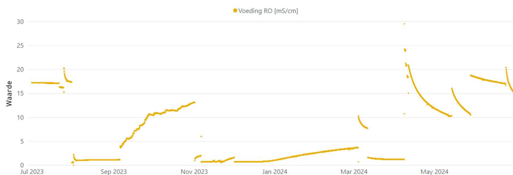
Figure 4.6: The conductivity in mS/cm of the influent water of the RO in the reporting period.
